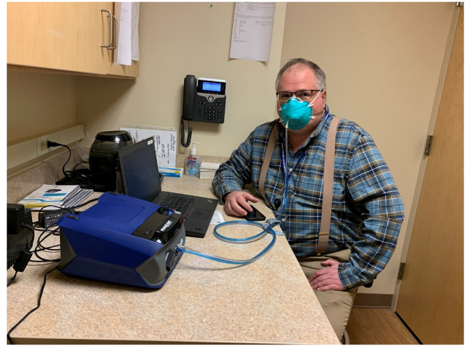
Fig. 7. Fit testing N95 mask with PortaCount®.
