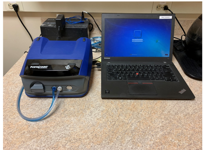
Fig. 8. Portacount® quantitative fit test device.
