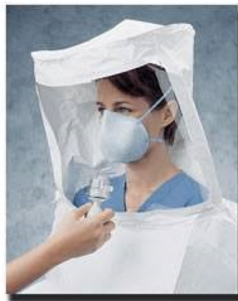
Fig. 4a. fit testing N95 mask with qualitative solutions (isoamyl acetate, saccharine, etc.).
